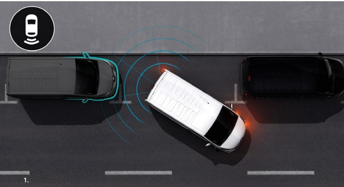
**1. Rear parking sensor:** To facilitate parking manoeuvres, the parking aid alerts you to any obstacles behind the vehicle with an audible signal. You can then reduce the risk of accidents and damage to your vehicle.
